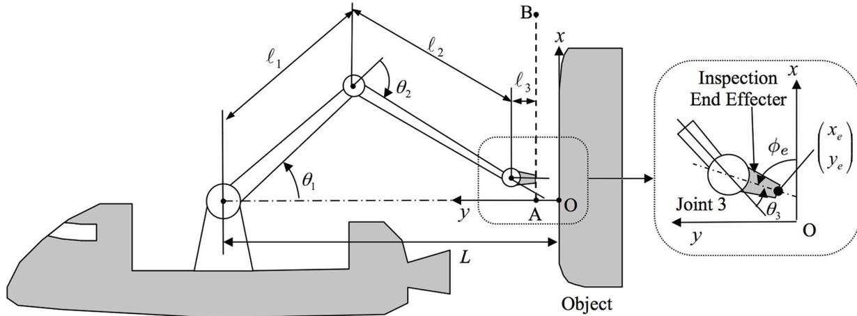
Figure 2: Shuttle manipulator inspecting an object surface. Note: All the angles are measured in the right hand sense, i.e.,  $\theta_2$  as depicted in the figure is negative.
