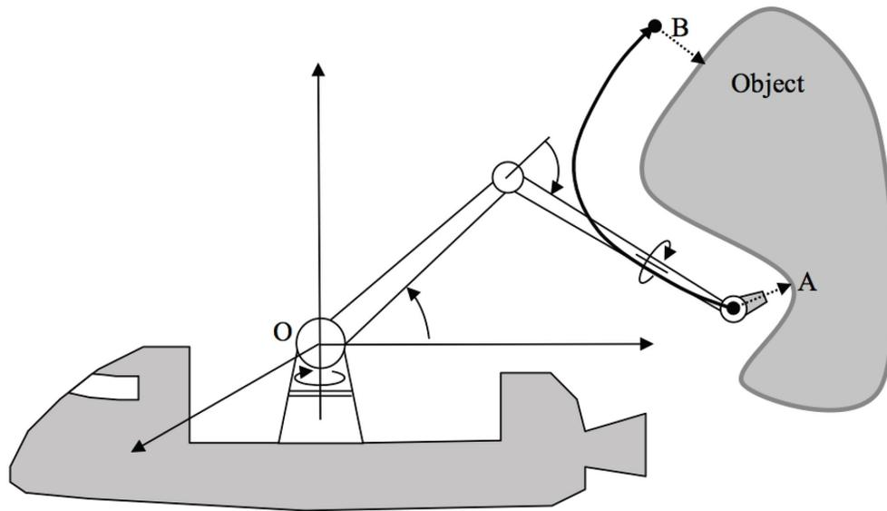
Figure 4: Space Shuttle manipulator tracking a curved surface.
