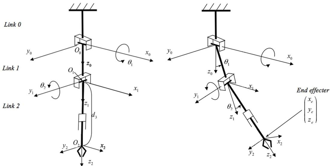
Figure 1: Left: Home Position. Right: Configuration  $(\theta_1 = \pi/6, \theta_2 = \pi/6, d_3 = 20 \text{ cm})$ .
