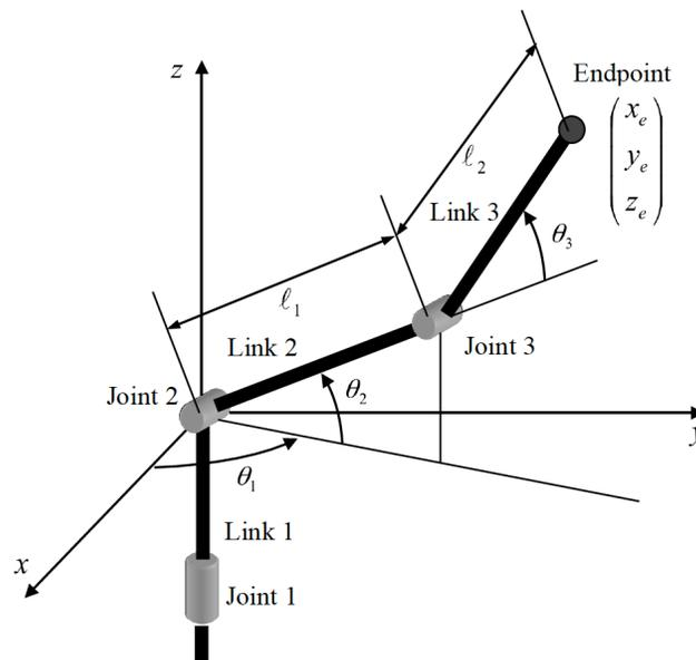
Figure 1: Schematic of a three dof articulated robot.
