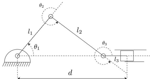
Figure 2: Slider Crank Mechanism.
