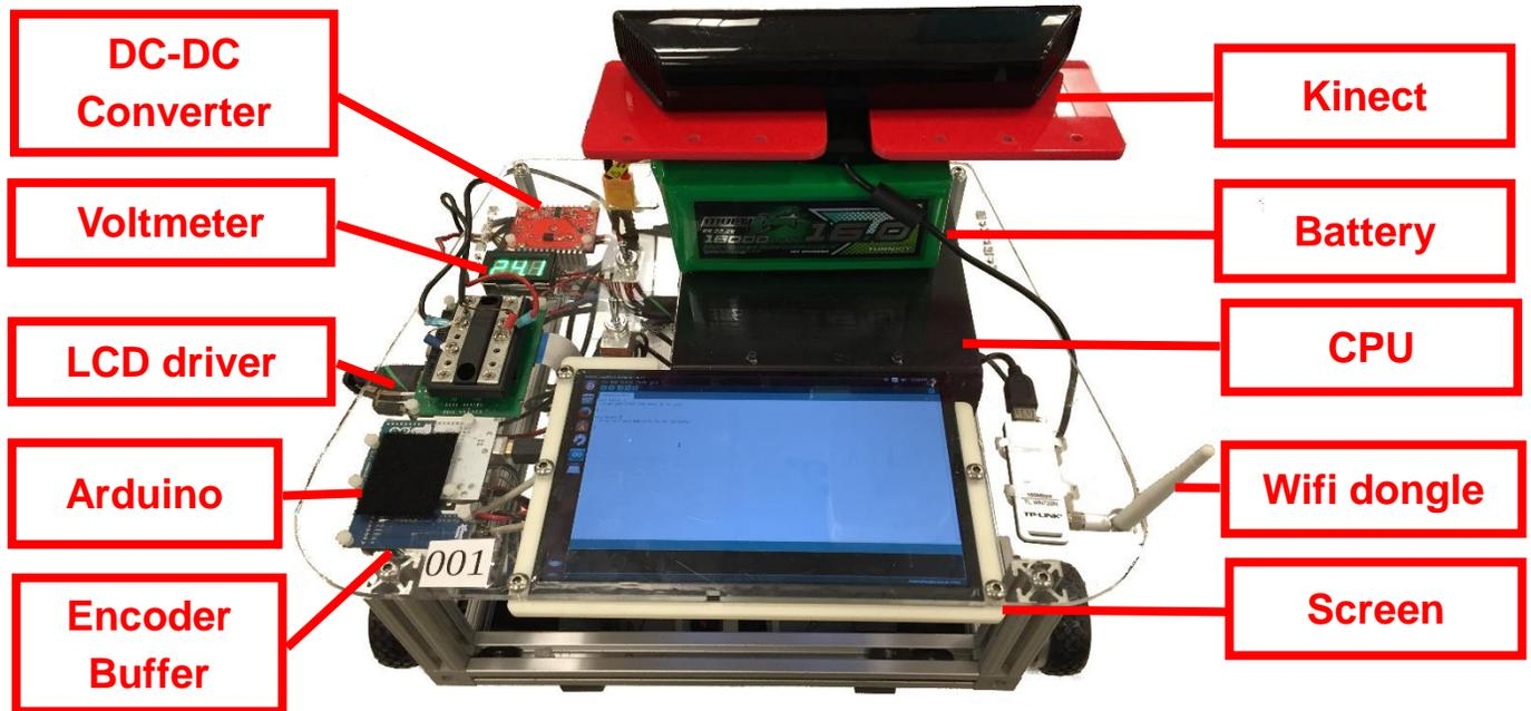
Figure 1: Our mobile robot platform.
